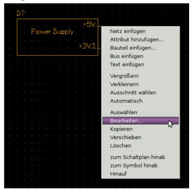
add attribute "source" with the value "powersupply.sch" and place the attribute below the symbol in the schematic
